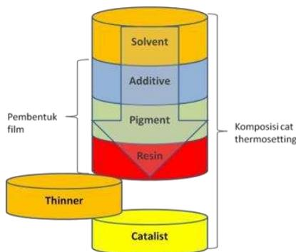
**Gambar 10.** Komposisi material cat jenis *polyurethane (thermosetting)*
