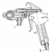
**Gambar 5.** Manual Spraygun (1. Paint supply, 2. Compressed gas supply)
