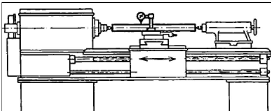
**Gambar 6.** Metode Pengujian Kelurusan sumbu antara *head stock (axis of centres parallel with bed in vertical plane)*; (Sumber: Georg Schlesinger, 1970, pp 53)
