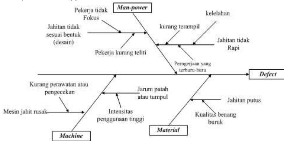
Gambar 4. Diagram fishbone cacat (*defect*)
