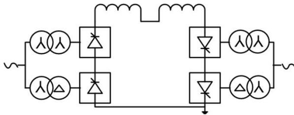
Figure 2: Monopolar HVDC with metallic return
