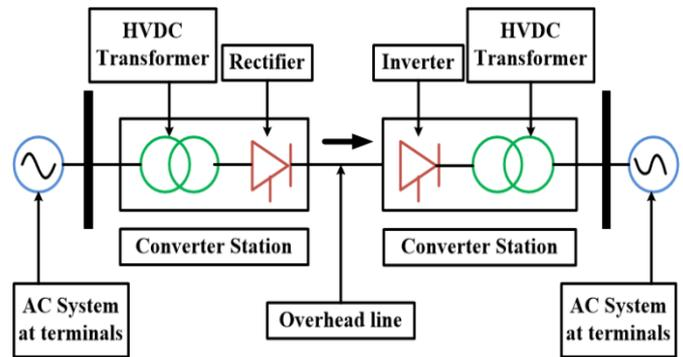
Figure 4: Typical layout of a HVDC link
