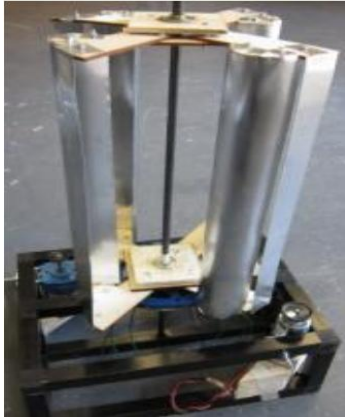
Figure 1: Vertical Axis Wind Turbine- Savonius type [1]
