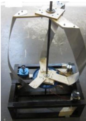
Figure 2: Vertical Axis Wind Turbine- Darrieus type [1]
