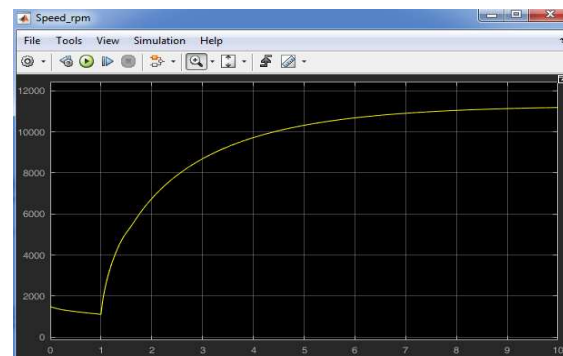
Fig. 15: Speed of SEIG at 6.6 KW load
