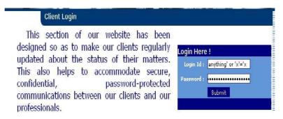
This injection is successful as it logged on to the account of a client of the company; so even this simple code can cause trouble.
