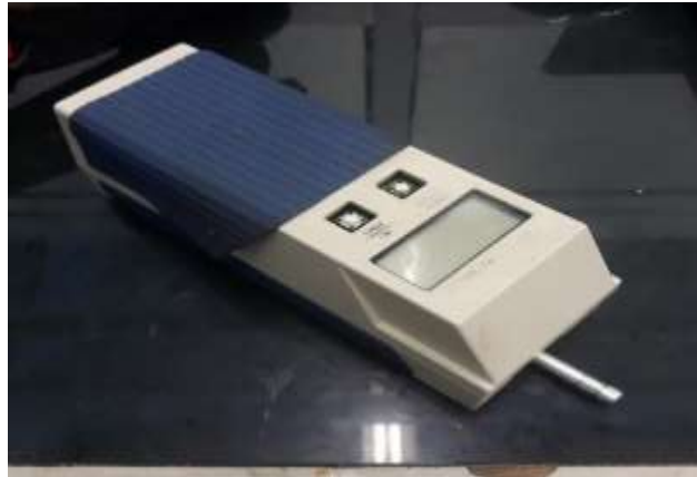
Figure 3. Surface Tester Mitutoyo 211
