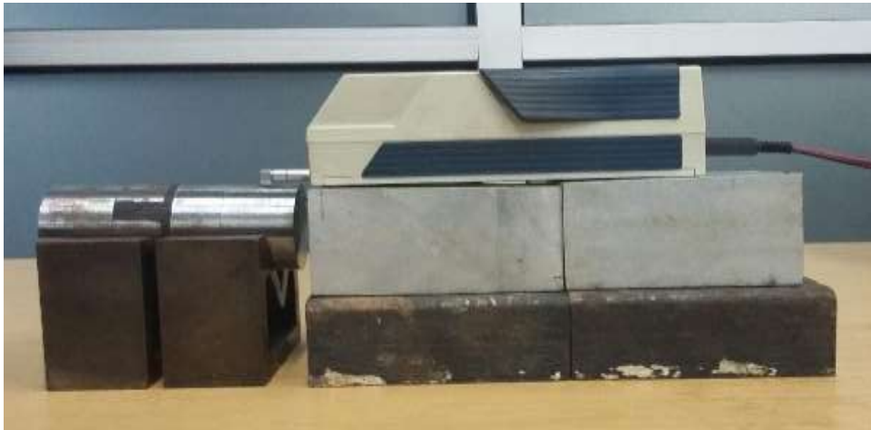
Figure 5. Surface Roughness Measurement
