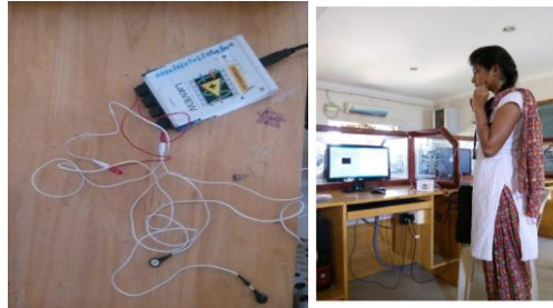
Figure 2. Surface electrode with NI-DAQ and measurement of the input signal
