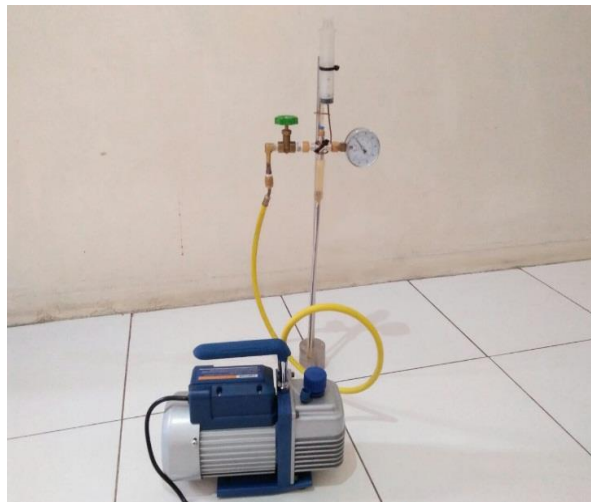
Gambar 4. Proses vakum pipa kalor
