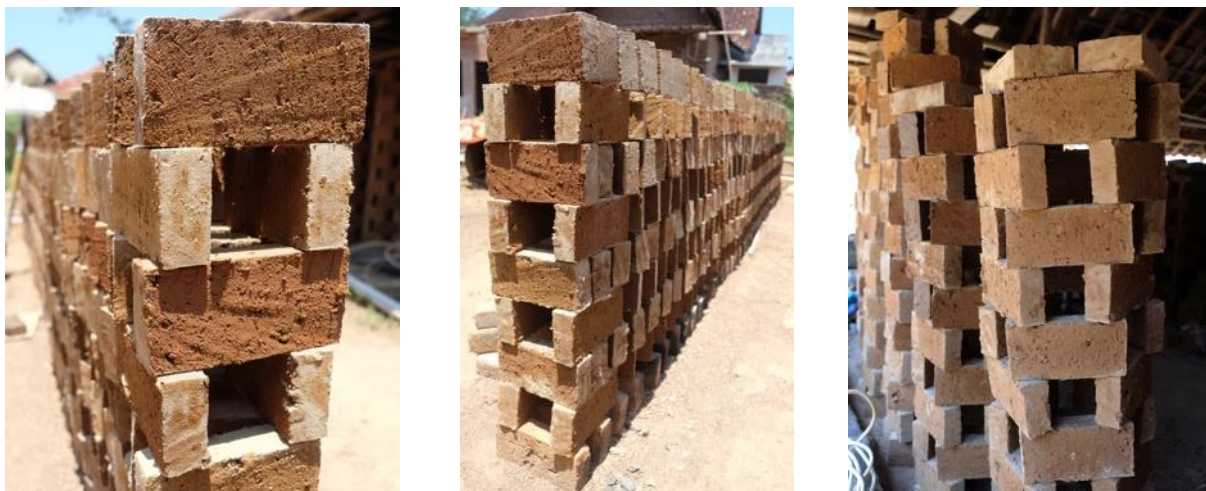
Figure 3. A pile of sun-dried clay bricks.
