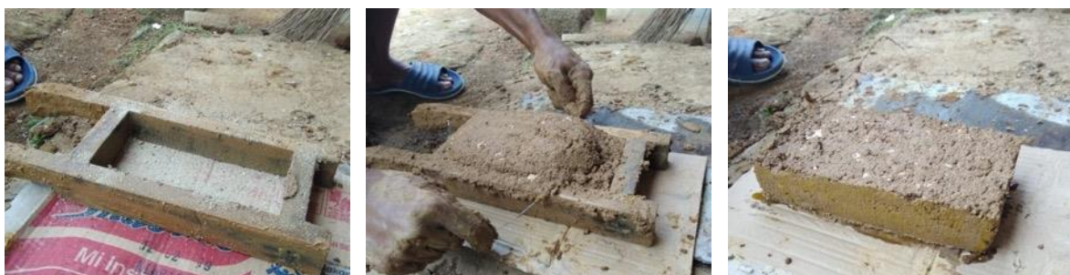
Figure 1. Manual moulding with a wood block and a wire.
