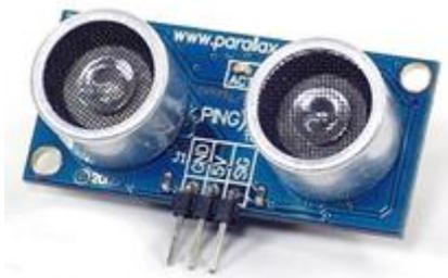
**Gambar 1. Sensor Ultrasonik**
