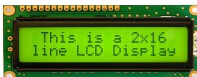
**Gambar 3. LCD 16x2**
