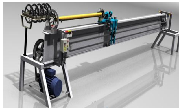
Figure 4. Proposed technology for the cutting and chipping of guadua cane
