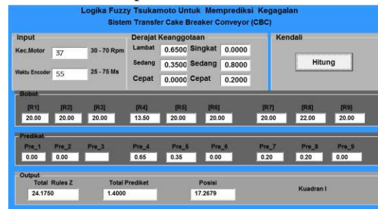
Gambar 8. Software aplikasi deteksi kegagalan system transfer cake breaker conveyor.
