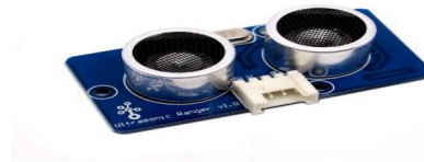
Gambar 2. Sensor Ultrasonik HC-SR04 (Sumber: http://www.seeedstudio.com )
