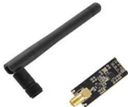
Gambar 3. Modul Transceiver bRF24L01.
