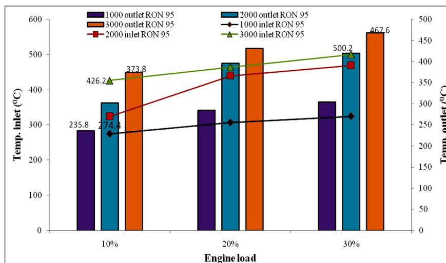
Figure 6. Exhaust gas temperature inlet and outlet of FeCrAl CATCO fuelled by RON 95
