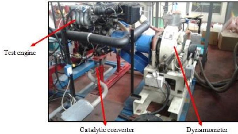
Figure 2. Mitsubishi 4G93 engine with eddy current dynamometer
