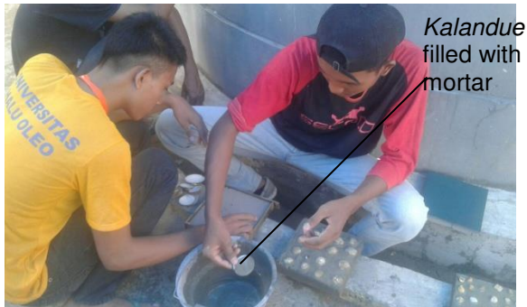
Figure 3. Kalandue shell filled with mortar
