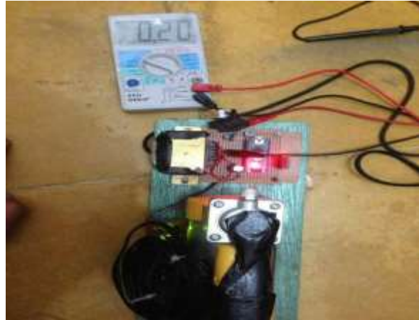
Figure 10. Results of Voltage Measurement on MPX 5500 Pressure Sensor
