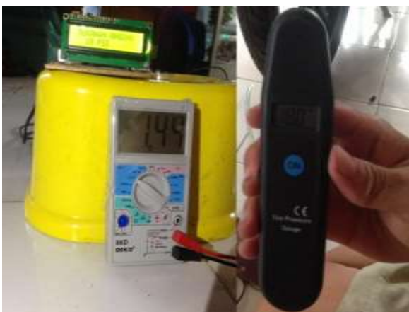
Figure 9. (c). The results of the comparison between the TPMS Prototype and the Digital Tire Pressure Gauge Tool worth 18 PSI
