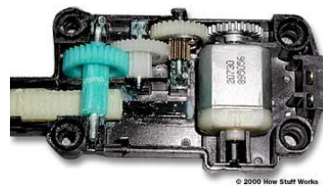
Gambar 10. Susunan Gearbox Central Lock Arduino Mega 2560
