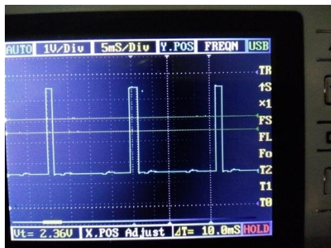
Gambar 14. Duty Cycle PWM 25bit
