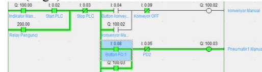
Gambar 28 Tampilan Ladder Saat Button Valve "HIGH"
