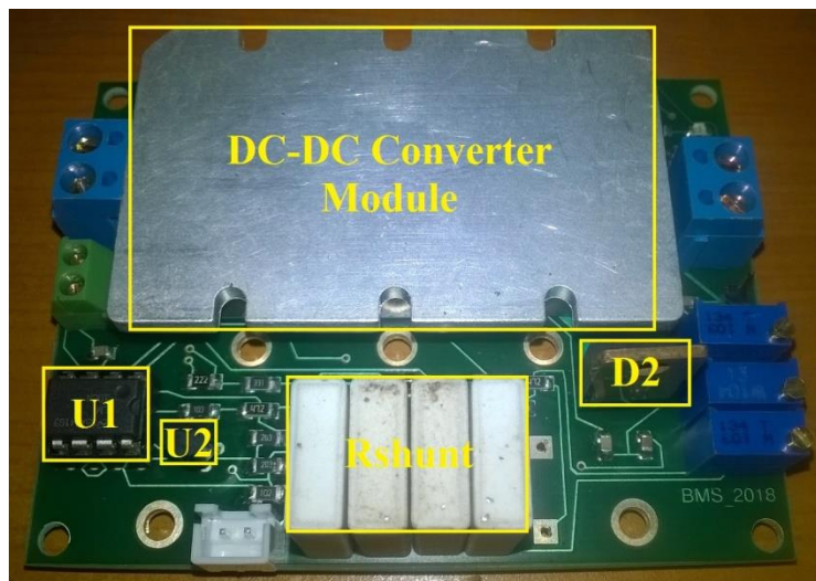
Figure 4. LiFePO 4 battery charger prototype
