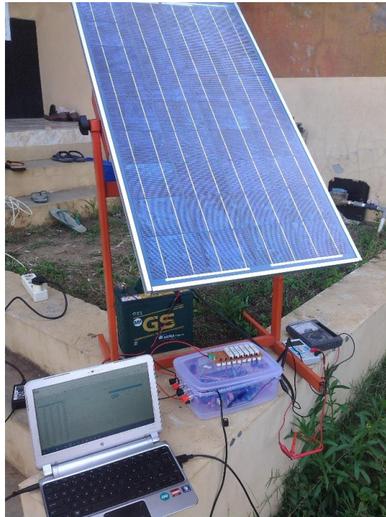
Figure 9. Implementation of MPPT on location
