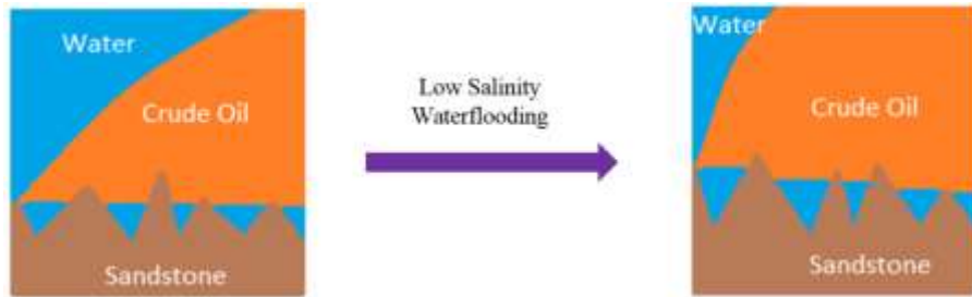
Figure 8 Illustration of surface roughening effect after low salinity waterflooding. The enhanced surface roughness leads to a more water-wet system.
