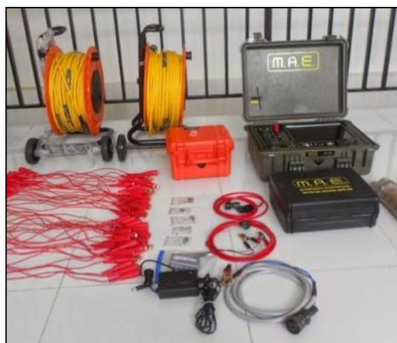
Gambar 3. Alat ukur resistivitymeter multichannel MAE X612EM+.
