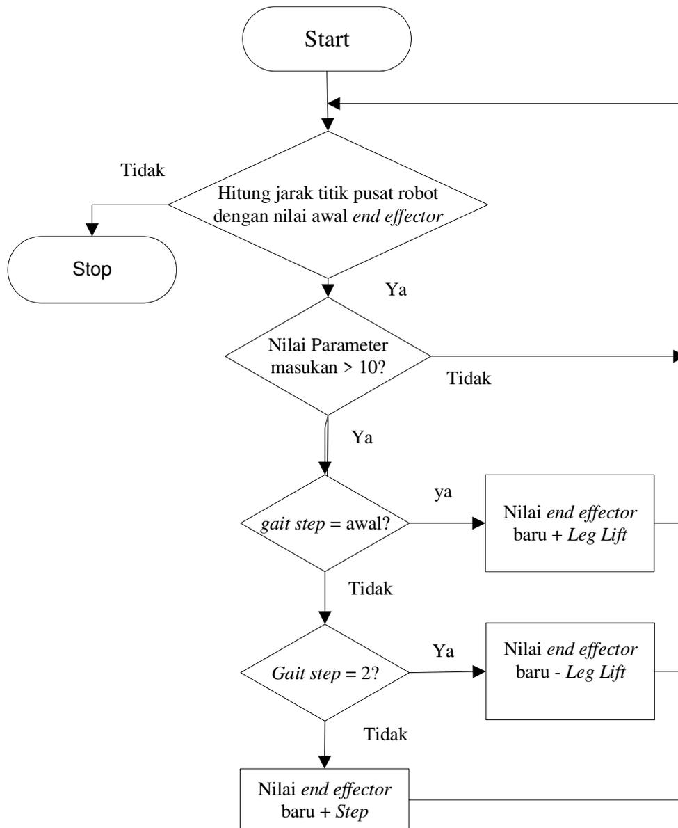
Gambar 11 Diagram alir program algoritma *gait*
