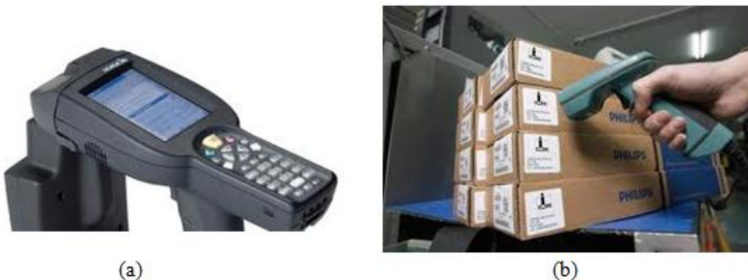
■ Gambar 15. Handheld RFID reader, (a) unit handheld, (b) proses pemindai barang.
