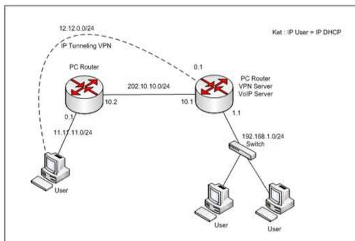
■ Gambar 3. Desain Prototype VoIP over VPN
