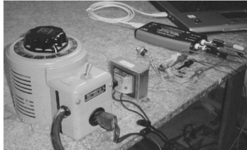
■ Gambar 2. Curve Tracer Berbasis PC
