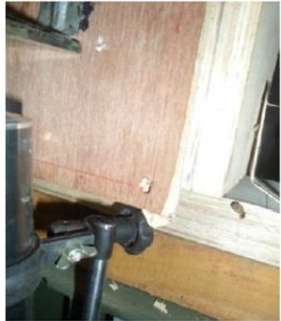
(a) Nail Pull-Through of Sheathing
