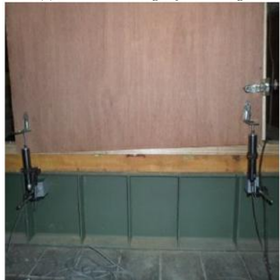
(b) Pull-Through Sheathing Failures
