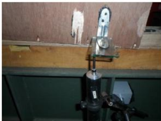
(c) Nail Pull-Through of Sheathing
