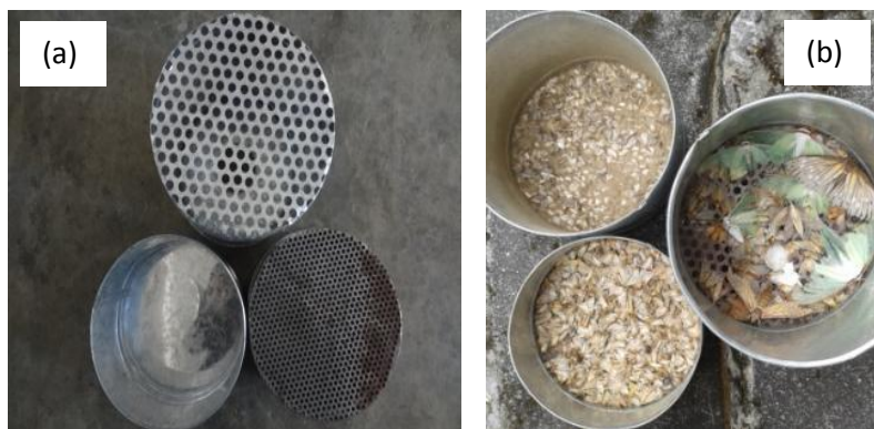
Fig. 4. Insect collection chamber (a) sieve at bottom of collection chamber (b) insects sorting in different chambers
