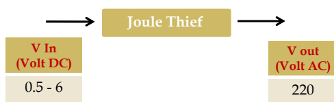
Gambar 7. Blok Diagram Joule Thief
