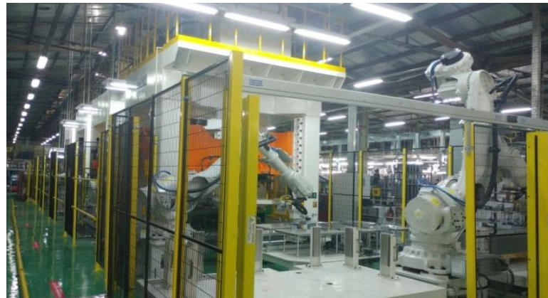
Figure 3 Layout automation out door forming process by robots.
