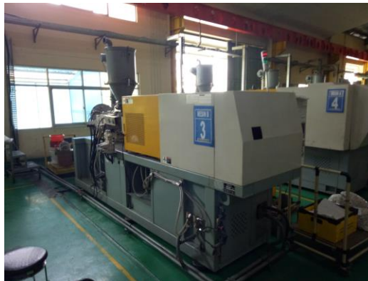
Figure 3. Injection molding machine Toshiba IS 350 GS 350 Ton
