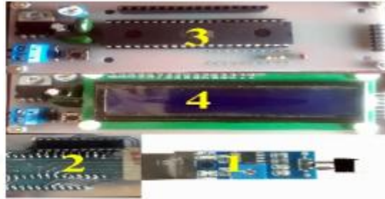
Figure 2. Meat moisture measuring instrument with AT89S52 microcontroller based copper electrode sensor
