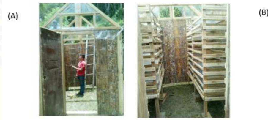
Figure 1. Solar drawer dryer
