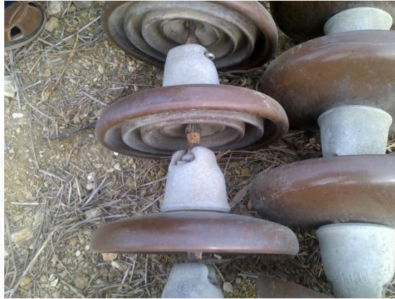
Figure 3. Sample of insulators deteriorated due to contamination
