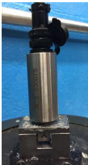
Fig. 2: Sensor mounted on shaker
