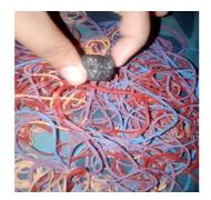
c. The next prosess was covering the plastic with rubber, then forming by coating some rubber to become a rubber ball of 6 diameters
