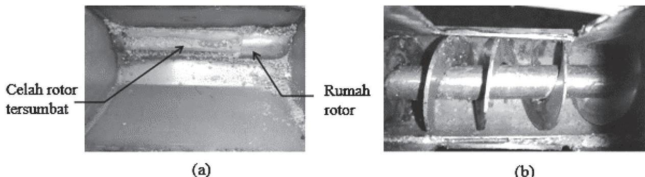
Gambar 10. (a) *Metering device* tipe *edge cell* (Sitorus, 2015); (b) *metering device* tipe *auger*.
