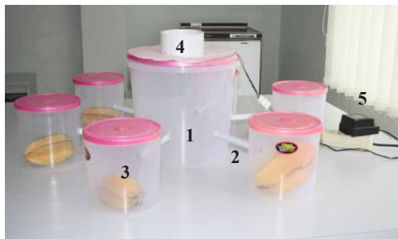
Figure 1. Wind tunnel front view. 1: fruit flies cage; 2: air canal pipe; 3: host fruit jar; 4: exhaust van; 5: adaptor.
