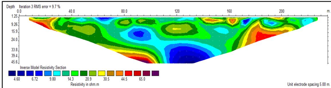
Figure 6. Geoelectrical cross section
