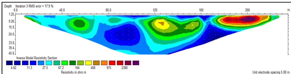
Figure 5. Geoelectrical cross section
