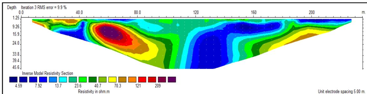
Figure 7. Geoelectrical cross section
