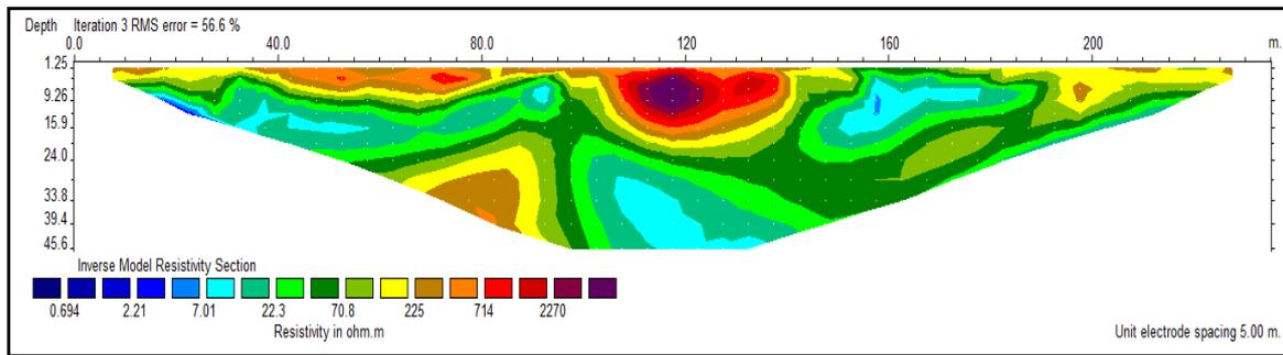
Figure 8. Geoelectrical cross section
