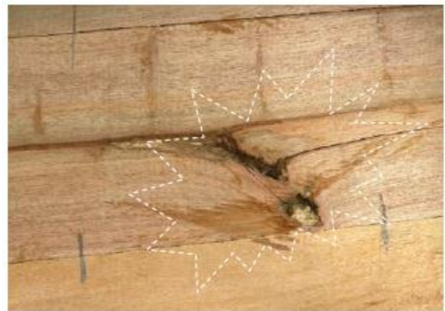
Gambar 5. Face knot and shake
