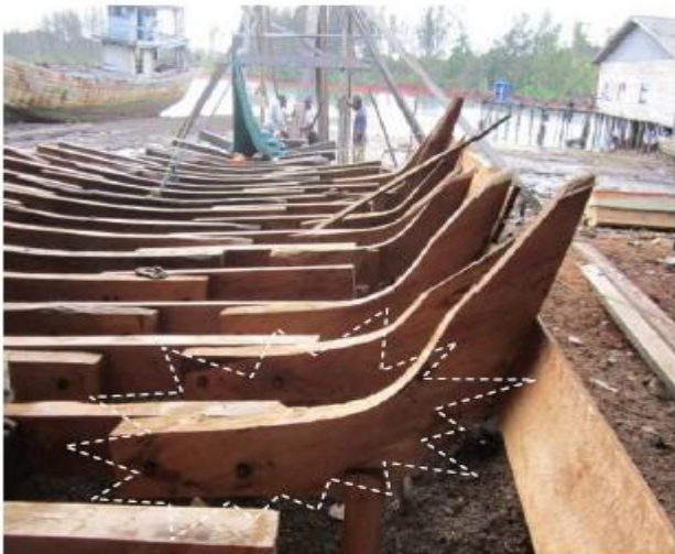
Gambar 3. Face knot on the bottom futtock ship
