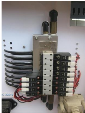
Gambar 10. 5/2 Single Solenoide Valve
