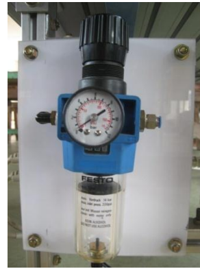
Gambar 11. Air Supply Unit
