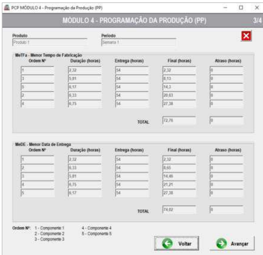
Fig. 7: Third screen of PPC software prototype of PS module.
