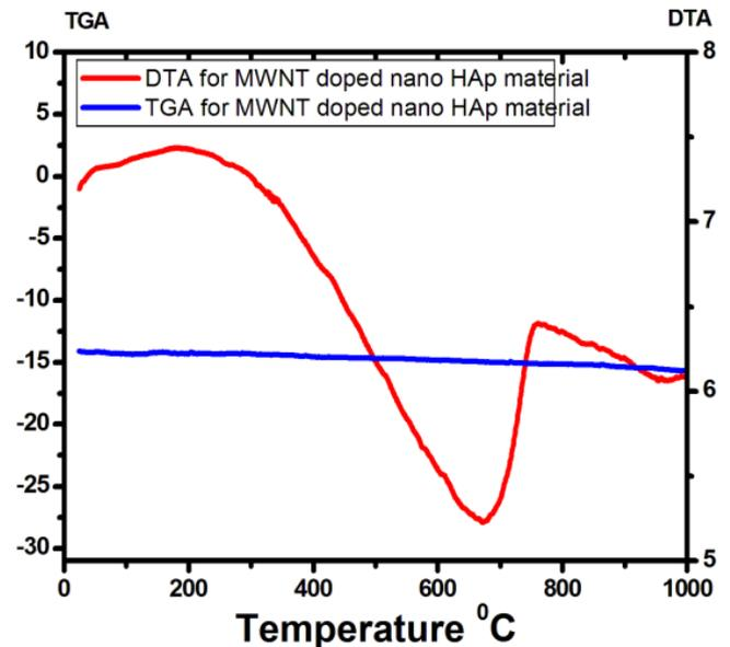
Fig. 4 Thermo- Gravimetry / Differential Thermal Analysis showing mass reduction due to heating for (a) MWNT powder showing thermal stability up to  $550^\circ\text{C}$  and (b) 0.2wt% MWNT doped nano-HAp composite showing high thermal stability ( $1000^\circ\text{C}$ ) for nano-HAp.
