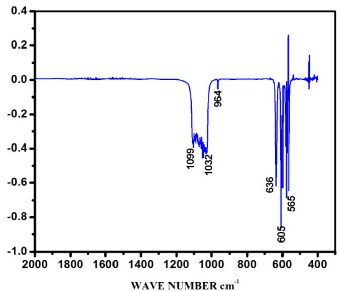
Fig. 5 FTIR spectra for MWNT doped nano-HAp composite material showing characteristics absorption peaks of the material as, hydroxyl liberation mode at  $636\text{ cm}^{-1}$ , phosphate band present in the range  $1000\text{ cm}^{-1}$  to  $1100\text{ cm}^{-1}$ ,  $\nu_1$
