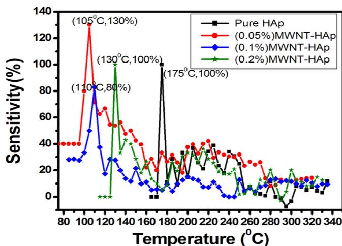
Fig. 6 Sensor sensitivity evaluated as the ratio of  $(R_g - R_a)/R_a$  v/s temperature for nano-HAp and MWNT doped nano-HAp composites sensor substrate to determine functional temperature in presence of 20 ppm CO gas.
