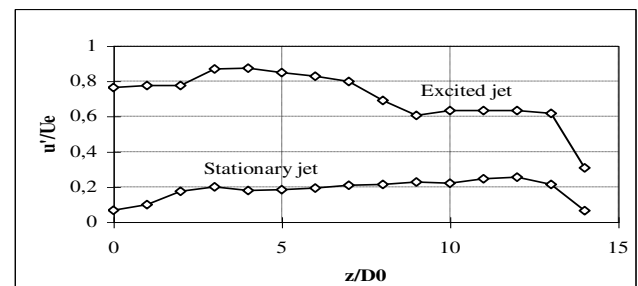
Fig. 10: turbulence intensity (for the axial velocity component) along the jet axis, as a function of the distance from the efflux.
