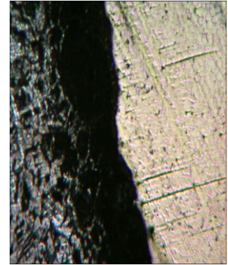
Figure 4: fusion boundary on 200 X magnification
