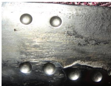
figure 2: hardness tested work piece
