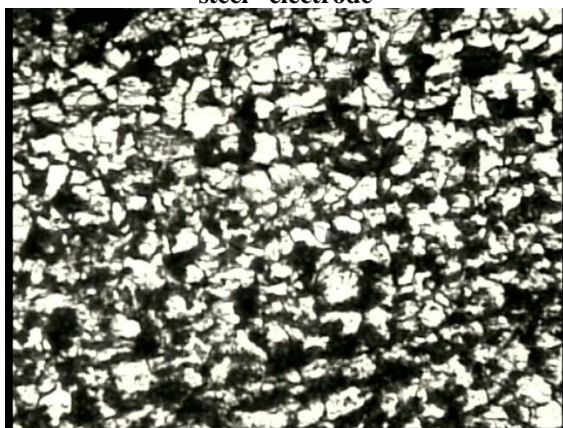
Fig6: unaffected zone by using mild steel filler and mild steel electrode
